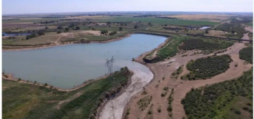
Figure 3. Ark River bank breach upstream of Garden City.
