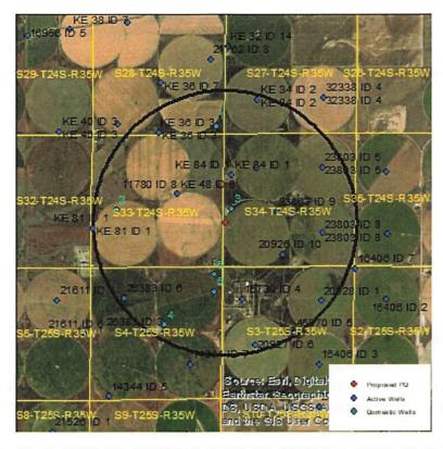
Wells within 1 mile: KE 84, 23803 ID5, 23803 ID6, 23803 ID8, 23803 ID9, 20926, KE 36, KE 34, KE 48 & 11780, 26383, 15730, 20927, 20928, 45870, and six domestic wells, numbered on the above map.
